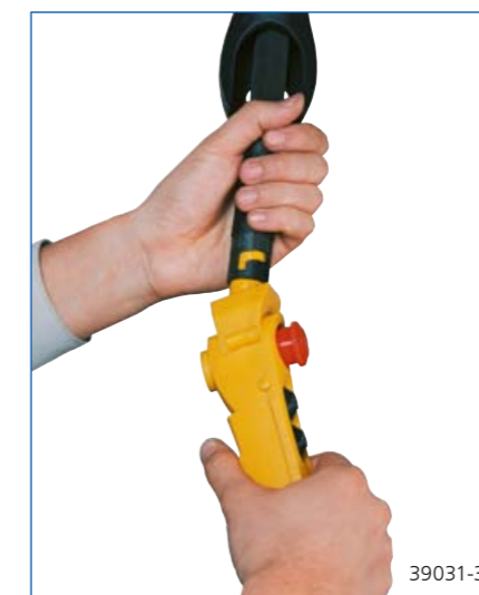
Fit the plug with its bayonet connector into the control pendant and turn until it locks
