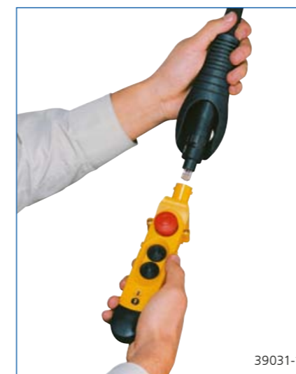
Slide the protective sleeve upwards over the control cable
