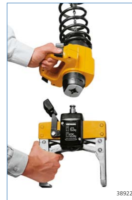
The quick-change coupling on the DSM-C control unit
